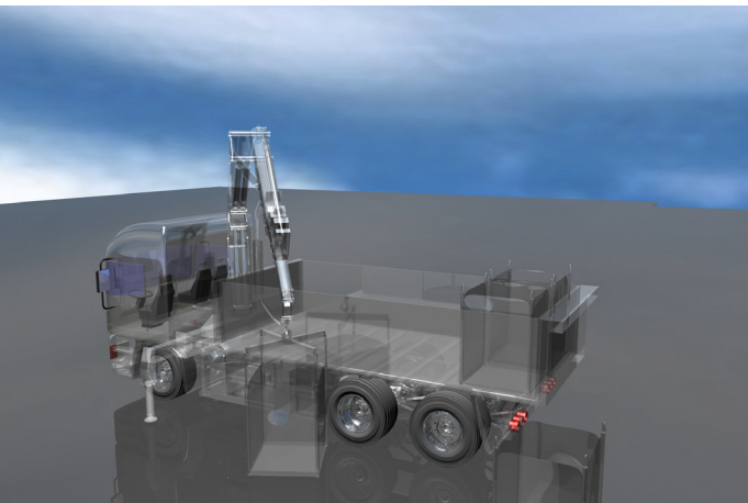
Truck mounted loading cranes are today powered by the diesel engine. On the other hand, the electro-hydraulic power take-off “eh-PTO” of an electrified truck, is connected directly to the battery.
